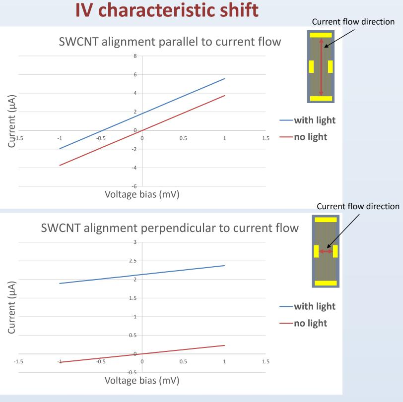
Resistance effects from large electrode distance overruled by effects of CNT alignment
